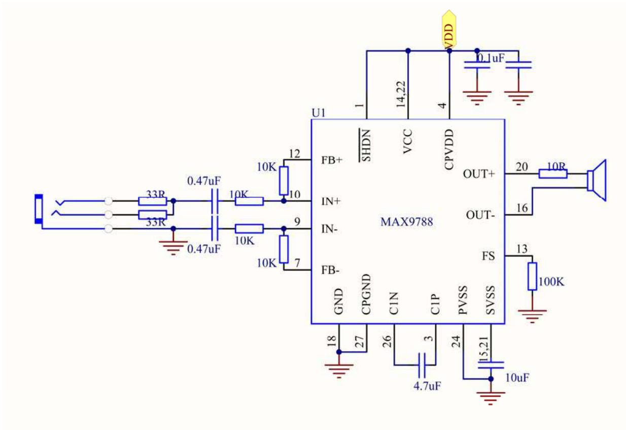
8. 5 The Voltage for above recommended circuits are under low 2.7-5.5V. If working under voltage, please refer to other desgins.
