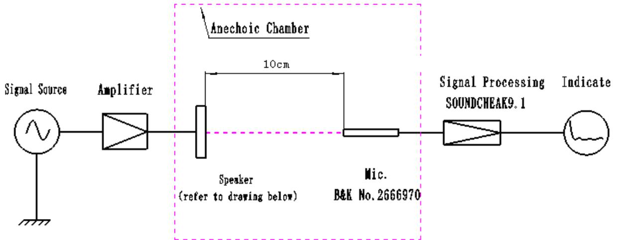
The speaker, being tested in an anechoic chamber, is installed in a baffle of 135cmx165cm.
